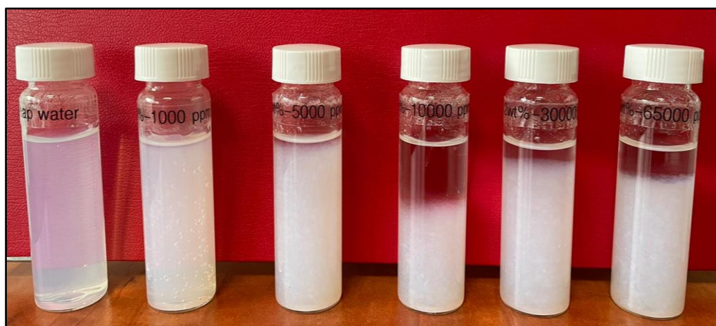
Figure 4.14: Solubility bottle tests for 2 wt% nanocellulose prepared by using water with varying salinities (after 6 hours at 65 °C)
