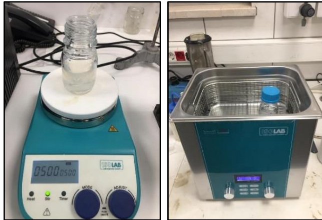
Figure 5.1: Preparation of diluted nanocellulose (stirrer on the left, sonic bath on the right)
