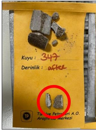
Figure 6.39: Samples used for after oil recovery test with 2 wt% nanocellulose (core plug #347)
