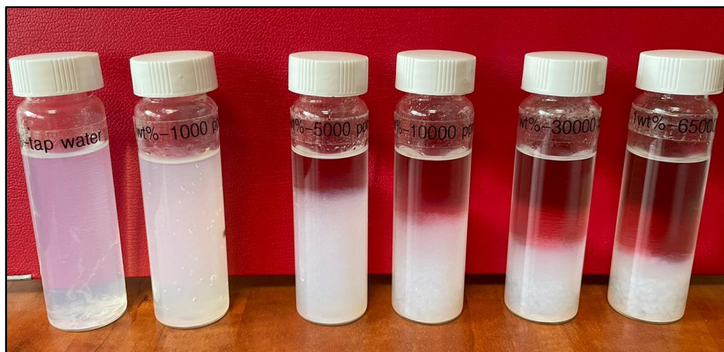
Figure 4.13: Solubility bottle tests for 1 wt% nanocellulose prepared by using water with varying salinities (after 6 hours at 65 °C)
