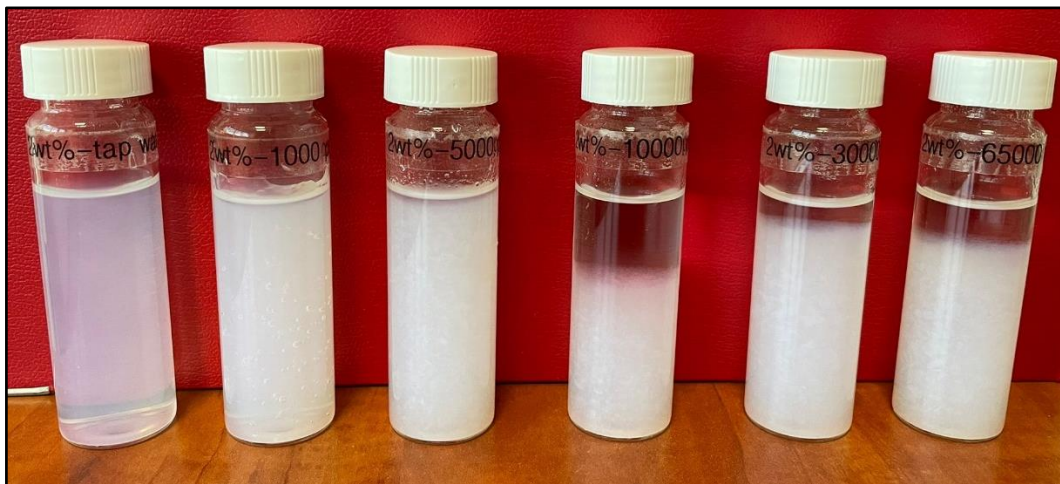
Figure 4.12: Solubility bottle tests for 2 wt% nanocellulose prepared by using water with varying salinities (room temperature)
