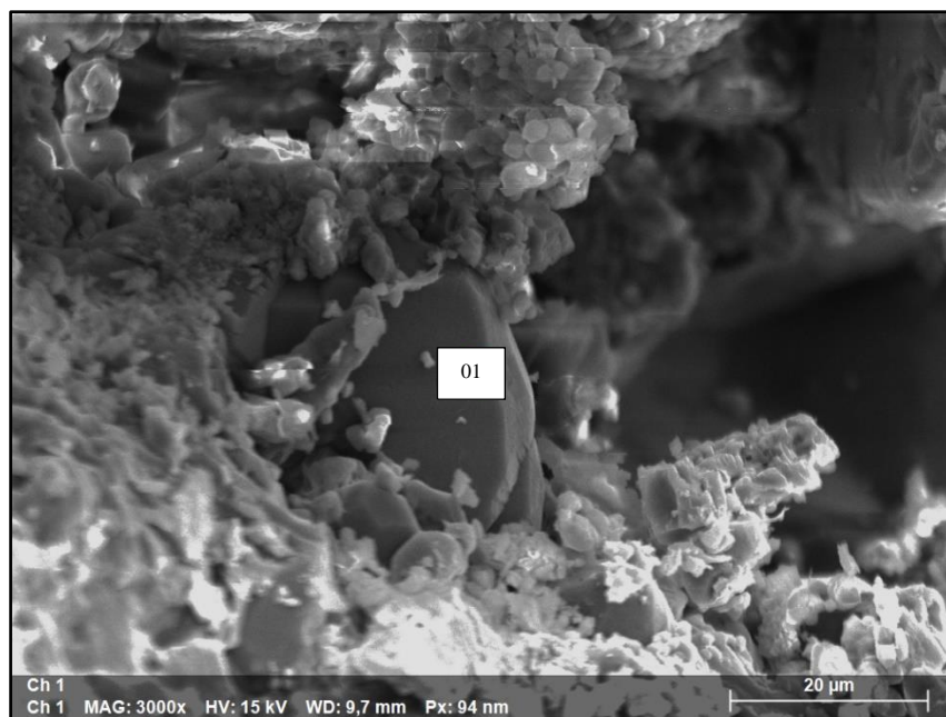
Figure 6.44: SEM image-1 of core sample #347 (sample in the right in Figure 6.39) after oil recovery test with 2 wt% nanocellulose
