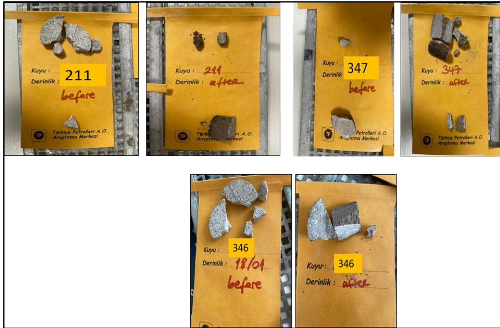
Figure 6.33: End trim samples of core plug 211, 347 and 346 before and after oil recovery coreflood tests
